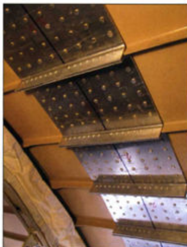
FAR LEFT The two fuselage cuts, now filled and rubbed down, are just visible in this view of the port fuselage of 'BBDG, taken from the cabin door, as are the replacement leading edge sections. LEFT Holding the fuselage together at the cut points are these riveted aluminium repair plates. They were designed and installed by the team from Air Salvage International, the company which has been responsible for the dismantling and structural reassembly of the Brooklands Concorde.
